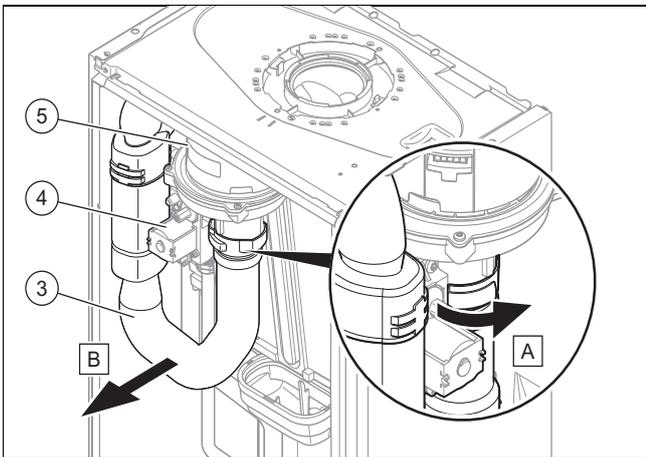
7. Remove the air intake pipe (3).
