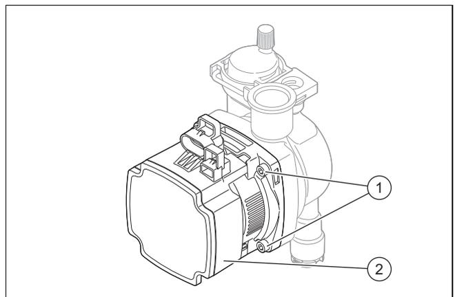
1. Disconnect the pump cables from the electronics box.
