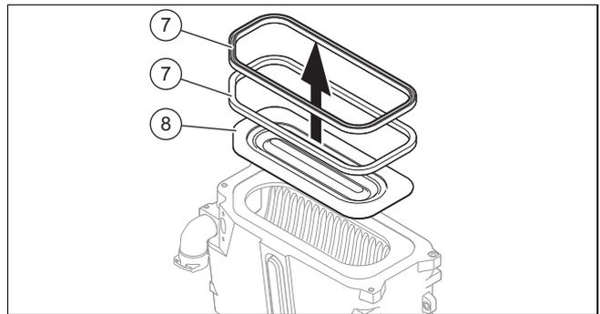
10. Remove the burner seals (7) and the burner (8).
