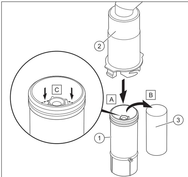
1. Unclip the lower section of the siphon (1) from the upper section of the siphon (2).
