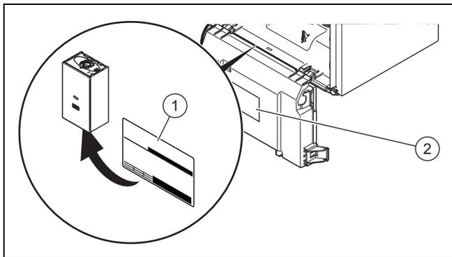
The serial number is located on the data plate (1).
