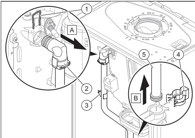
4. Remove the temperature sensor (3).
