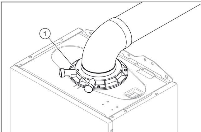
3. Unscrew the cover from the flue gas analysis point (1).
