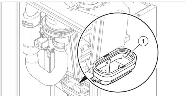
7. Using water to clean the condensate tray **(1)**.
