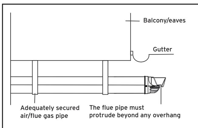
You can use a plume management kit to enable the termination point to be positioned and directed away from the building fabric.
