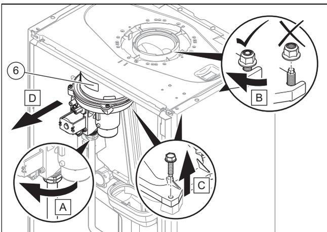
9. Remove the gas-air mixture unit (6).
