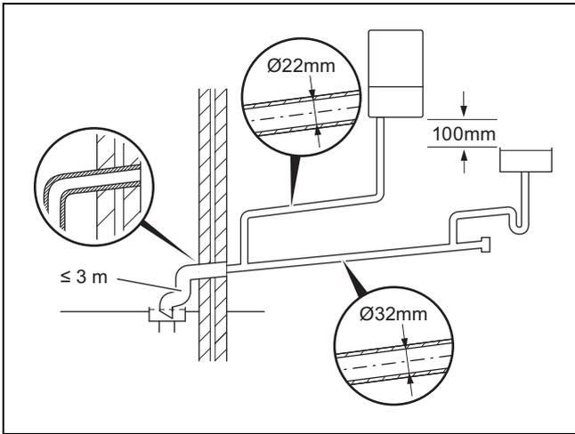
Open end of pipe direct into gully below ground level but above water level
