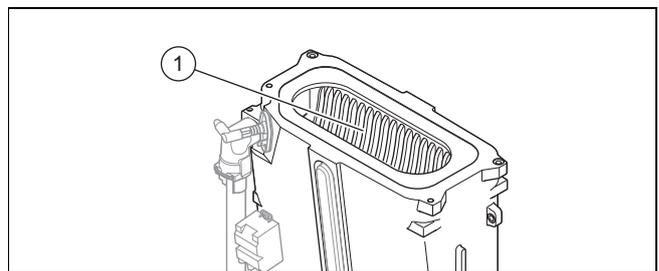
1. Protect the open electronics box from spraying water.
