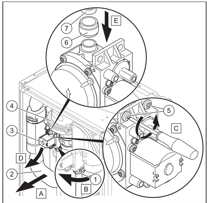
4. Remove the air intake pipe (2).
