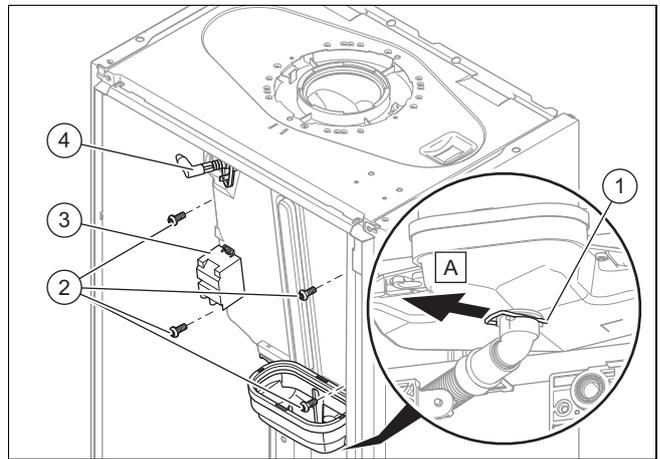
11. Remove the clip underneath the condensate tray (1).
